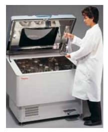
to 2 inches (5.1 cm). The size of the orbit will affect how the bacterial cells circulate and how the growth medium is aerated. It turns out that shaker orbit diameter has a linear relationship to the Oxygen Transfer Rate (OTR)<sup>4</sup>, which is the rate at which oxygen gas is transferred from the air to the liquid. Thus, if the orbital shaker diameter doubles, so does the OTR.
